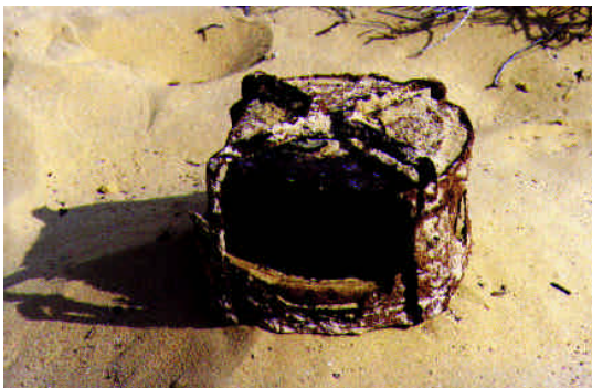
Photo: eg24-25a: Close up of Mk 5 AT mine showing advanced corrosion.
